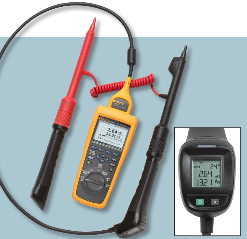
Intelligent test probe with integrated LCD display
