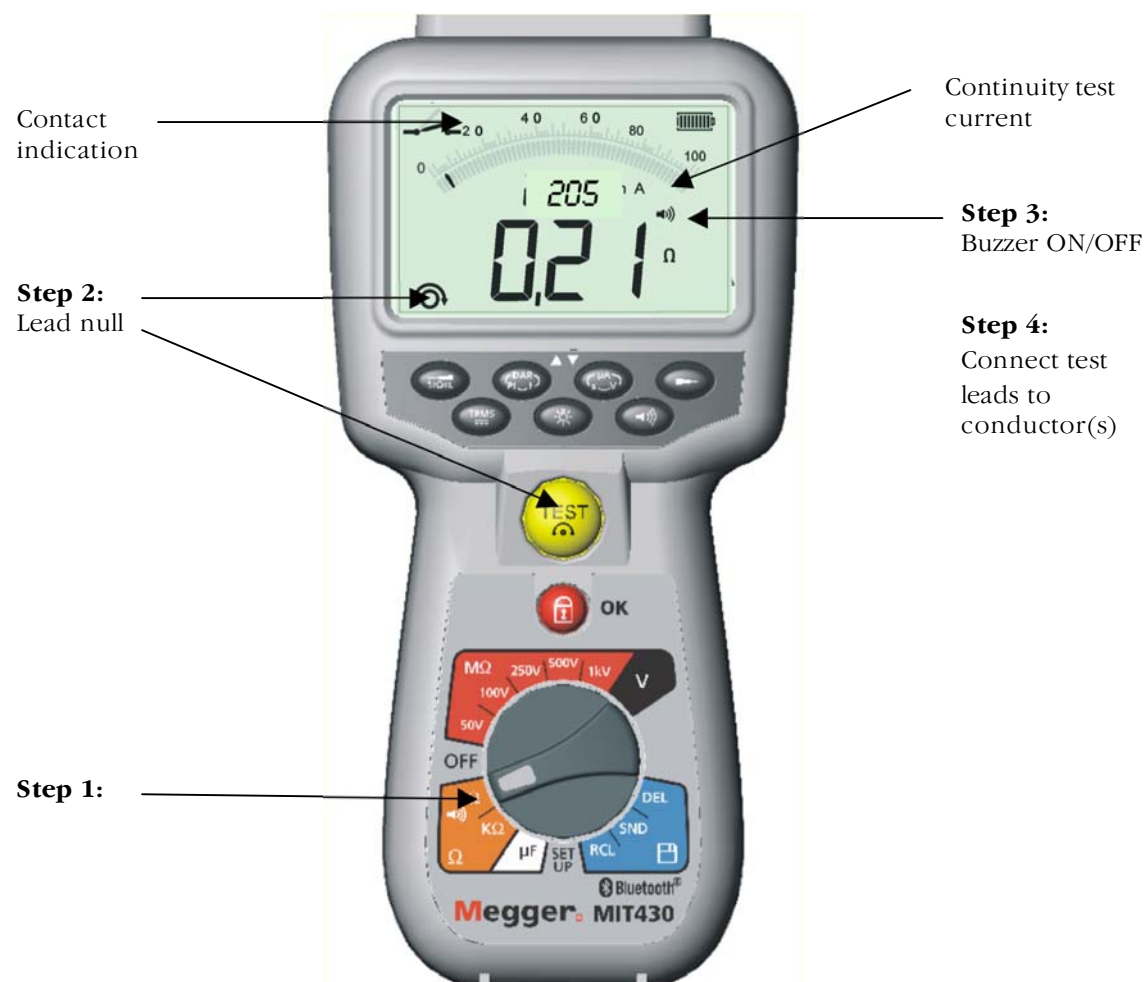
Figure 9 Continuity test and buzzer
