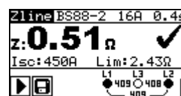
Figure 5.31: Examples of line impedance measurement result
