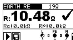
Figure 5.37: Example of earth resistance measurement result
