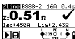
Figure 5.31: Examples of line impedance measurement result
