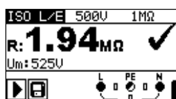
Figure 5.7: Example of insulation resistance measurement result
