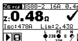
Figure 5.27: Examples of loop impedance measurement result
