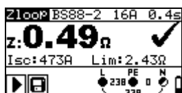
Figure 5.27: Examples of loop impedance measurement result
