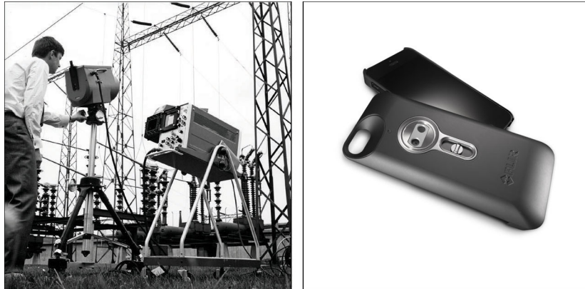
Figure 30.2 LEFT: Thermovision Model 661 from 1969. The camera weighed approximately 25 kg (55 lb.), the oscilloscope 20 kg (44 lb.), and the tripod 15 kg (33 lb.). The operator also needed a 220 VAC generator set, and a 10 L (2.6 US gallon) jar with liquid nitrogen. To the left of the oscilloscope the Polaroid attachment (6 kg/13 lb.) can be seen. RIGHT: FLIR One, which was launched in January 2014, is a slide-on attachment that gives iPhones thermal imaging capabilities. Weight: 90 g (3.2 oz.).
