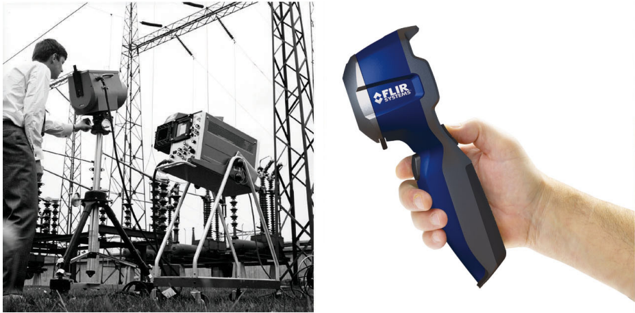
Figure 27.2 LEFT: Thermovision® Model 661 from 1969. The camera weighed approximately 25 kg (55 lb.), the oscilloscope 20 kg (44 lb.), and the tripod 15 kg (33 lb.). The operator also needed a 220 VAC generator set, and a 10 L (2.6 US gallon) jar with liquid nitrogen. To the left of the oscilloscope the Polaroid attachment (6 kg/13 lb.) can be seen. RIGHT: FLIR i7 from 2009. Weight: 0.34 kg (0.75 lb.), including the battery.
