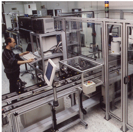
Figure 27.5 LEFT: Testing of infrared cameras in the climatic chamber; RIGHT: Robot used for camera testing and calibration
