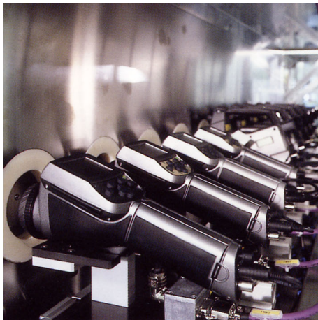
Figure 27.5 LEFT: Testing of infrared cameras in the climatic chamber; RIGHT: Robot used for camera testing and calibration
