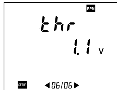
Figure 49: Display of parameter relating to the threshold voltage of the tachometer sensor.
