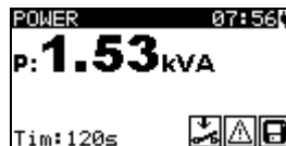
Figure 5.40: Example of apparent power measurement result
