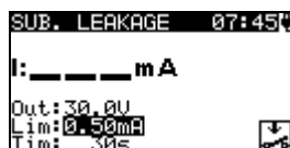
Figure 6.9: Substitute leakage starting screen
