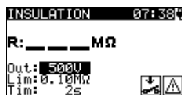
Figure 6.7: Insulation resistance starting screen
