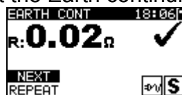
Figure 6.6: Earth continuity result screen
