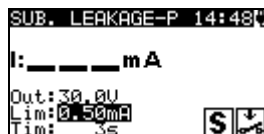
Figure 6.15: Substitute leakage - P starting screen
