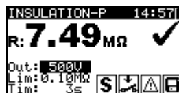
Figure 6.14: Insulation resistance - P result screen
