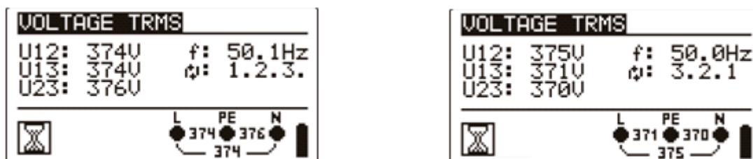
Figure 5.4: Examples of voltage measurement in three-phase system
