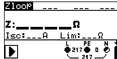
Figure 5.20: Fault loop impedance
