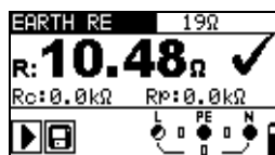
Figure 5.44: Example of earth resistance measurement result
