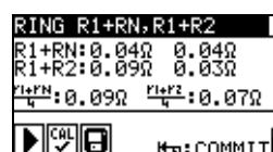
Figure 5.24: Examples of ring continuity test – step 2
