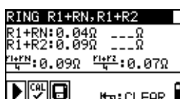
Figure 5.24: Examples of ring continuity test – step 2
