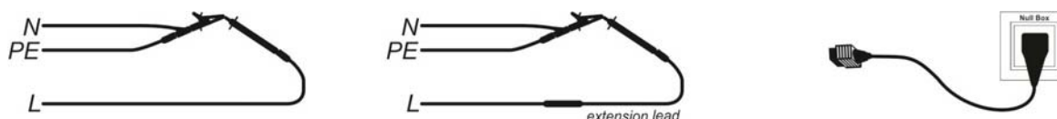
Figure 5.17: Examples of connections for compensation
