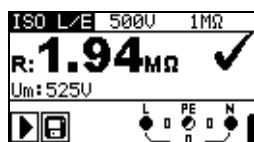
Figure 5.7: Example of insulation resistance measurement result
