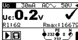
Figure 5.27: Example of contact voltage measurement results
