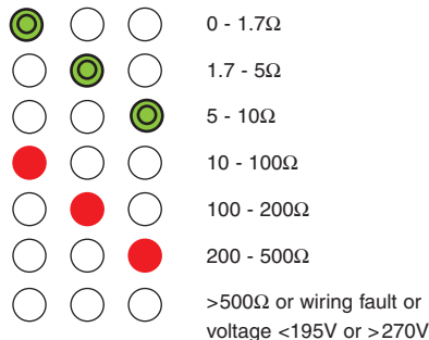
Figure 1. Loop Test (Top Indicators)
